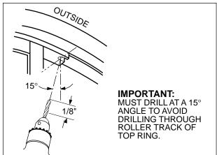
Drill a 3/32" diameter hole into the top ring at about 15°. (See Illustration 20.) Engage the top of the fixed panel with the top ring groove. Secure the top of the fixed panel to the top ring. (See Illustration 21.)
